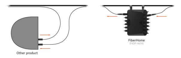
It can realize bothend in and out, more convenient for cable messenger installation
